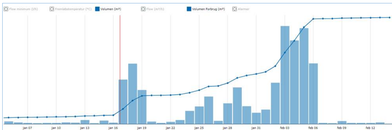
Figure 5: A local Supermarket gets mid-January a leak in the internal system. They receive a warning from BWC, and they fix the problem effectively two weeks later.
