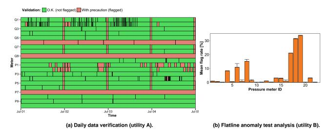
**Figure E-1.** Example of anomaly visualization for operational use. (a) Raw meter data validation from ten flow (Q) and pressure (P) meters in utility A in July 2015. (b) Mean flag rate based on all raw data points for the flatline test in pressure meters of utility B. Whiskers display the total flag rate based on all anomaly tests in the individual pressure meter.
