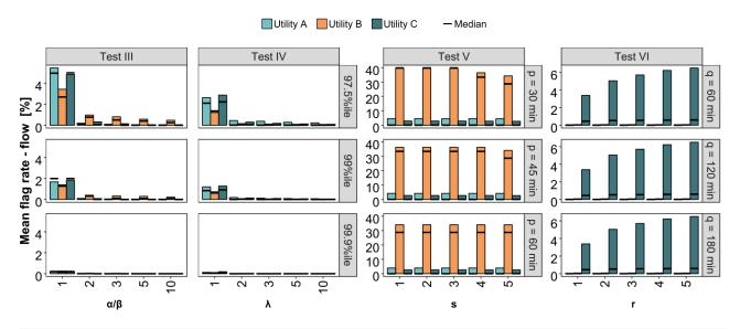
**Figure D-1.** Effect on error rates of all flow meters by varying test parameters on the range test (test III), change in rate test (test IV), flatline test (test V), and timestamp inconsistency test (test VI), based on the raw data from three utilities.
