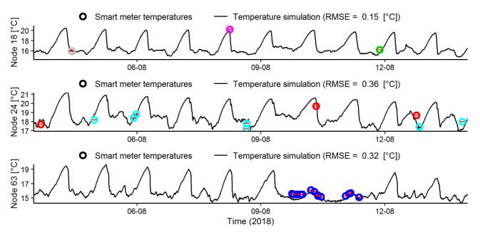
**Figure 8.** Smart meter temperatures (including  $\pm 1$  hr error margin) vs. simulated temperatures and the respective root mean squared error (RMSE). Distinct colours represent unique smart meters.
