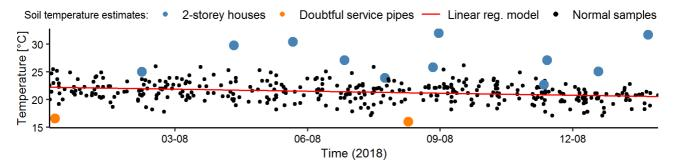
**Figure 5.** Soil temperature estimates and fitted linear regression model with anomalies (2-storey houses and doubtful service pipes) removed.
