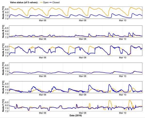
**Figure D-1.** Simulated water temperature in selected nodes of the DMA model with all valves open (orange) and five valves closed (blue).
