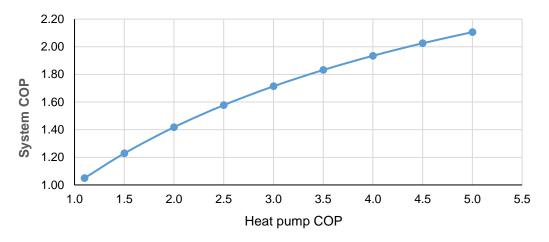
Figure 14. System COP vs. heat pump COP.
