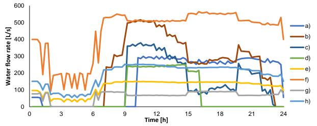
**Figure 5.** Daily water flow rates at the 8 selected heat pump locations. The flow rate during hours with changing direction have been set equal to zero since the heat pumps do not operate during this period. Three locations (e, f and h) have unidirectional flow for 24 hours. In order to avoid excessively cold temperatures, the operation of node d is particularly constricted since a part of its stream has already been cooled by another heat pump during several hours.
