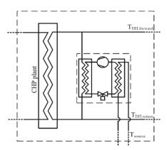
**Figure 3.** Configuration of heat pump connection to a DH line (from [29]). The heat pump increases the temperature of a part of the return flow ( $T_{DH,return}$ ) to the supply temperature ( $T_{DH,supply}$ ), via a reduction of the drinking water temperature ( $T_{source}$ ).
