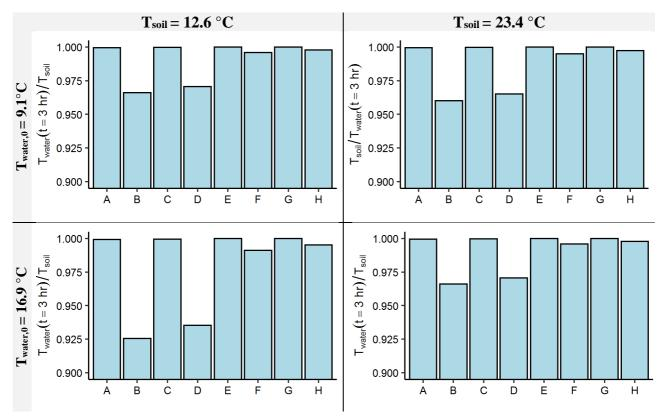
Figure A-2. Sensitivity analysis of parameters affecting the temperature in service pipes at t = 3 hr.
