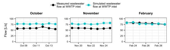
**Figure 3.** Observed ( $Q_{WWTP,obs}$ ) and simulated ( $Q_{WWTP,sim}$ ) wastewater treatment plant (WWTP) inflow in the three time periods.
