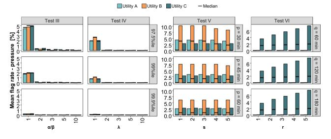
**Figure D-2.** Effect on error rates of all pressure meters by varying test parameters on the range test (test III), change in rate test (test IV), flatline test (test V), and timestamp inconsistency test (test VI), based on the raw data from three utilities.
