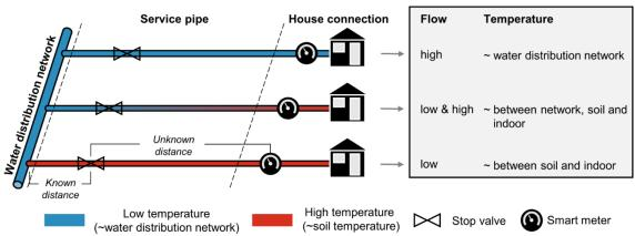
**Figure 9.** Variation in demand affects the residence time of the water in service pipes and house connections, leading to differing smart meter temperature measurements at the consumers' homes. Example from summer, with higher soil than water source temperatures.
