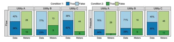
**Figure 5.** Summary of timestamp drift test. The data column accounts for the percentage of data where test condition 1 was met ( $C_{weekly}(d) \ge 0.8$ , for at least two reference weeks *w*). The meter column accounts for the number of meters meeting condition 2 at least once over the course of the measured period ( $|P_{weekly}(d)|>2$ , for more than two subsequent test days *d*).
