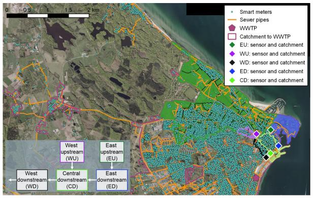
**Figure 1.** Map of Elsinore, Denmark, showing smart meters, the sewer system, five in-sewer flow observation locations with related sub-catchments (sub-divided into 111 smaller groups for smart meter aggregation), the wastewater treatment plant (WWTP), and the catchment discharging water to the WWTP. The flow between the sub-catchments in the sewer system is displayed in the lower left corner.
