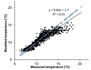
**Figure 7.** Modelled water temperatures vs. weekly measured temperatures (1497 samples from 15 sampling points). The blue dots represent the peripheral location used to determine the soil temperature.
