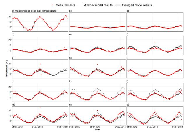
**Figure 17.** Measured and modelled water temperature data from 15 locations in Copenhagen from July 2012 to August 2014. Model averages are shown together with the minimum and maximum values obtained between 7 a.m. and 12 p.m.
