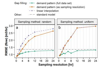
**Figure 5.** Root mean square error (RMSE) between measured inflow in DMA and accumulated demand in water distribution network simulations at various sampling resolutions and gap filling methods. The standard model represents a top-down approach where the same demand pattern was assigned to each node based on the consumption over 5 months.
