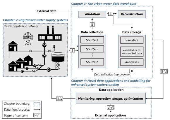
**Figure 3**. Conceptual overview of data flows in a water utility. The focus of each chapter is delineated by blue boxes.
