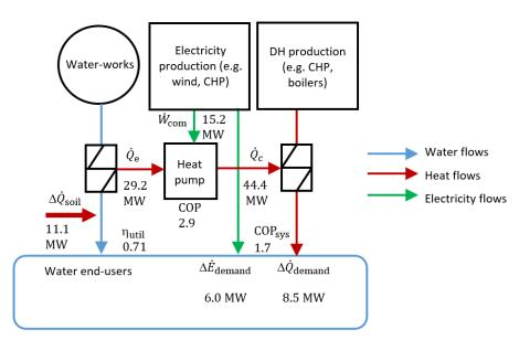
Figure 11. Change in the system energy flows resulting from a  $\Delta T_{source}$  of 5 K.
