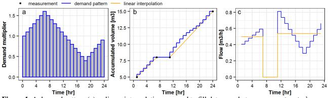
**Figure 1.** A demand pattern (a) or linear interpolation are used to fill data gaps between a smart meter's accumulated volume measurements (b), resulting in different flow rates over time (c).
