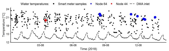
**Figure 6.** Water distribution network temperature estimates based on smart meter samples and the measured inlet temperature to the district metered area (DMA). Temperatures from two distinct nodes (44 and 64) resemble the bulk of temperature estimates, but differ highly when compared with simulated temperatures (Figure 7b).
