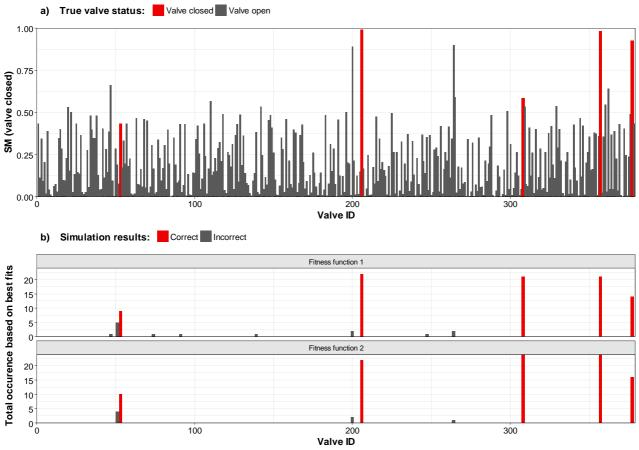
**Figure 6.** a) Similarity measure (SM) of a valve being closed (1) or open (0) used to compute an initial population. b) The total number of times a valve had been closed during the 24 GA runs of fitness functions  $F_1$  and  $F_2$ .
