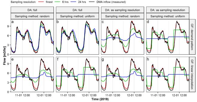
**Figure 4.** Example of simulated total consumption over two days in 2019 in DMA with varying sampling resolution, sampling methods and gap filling methods. For smooth illustration, a rolling mean window of 1 hour was applied to the data set. DA = data availability; GF = gap filling.
