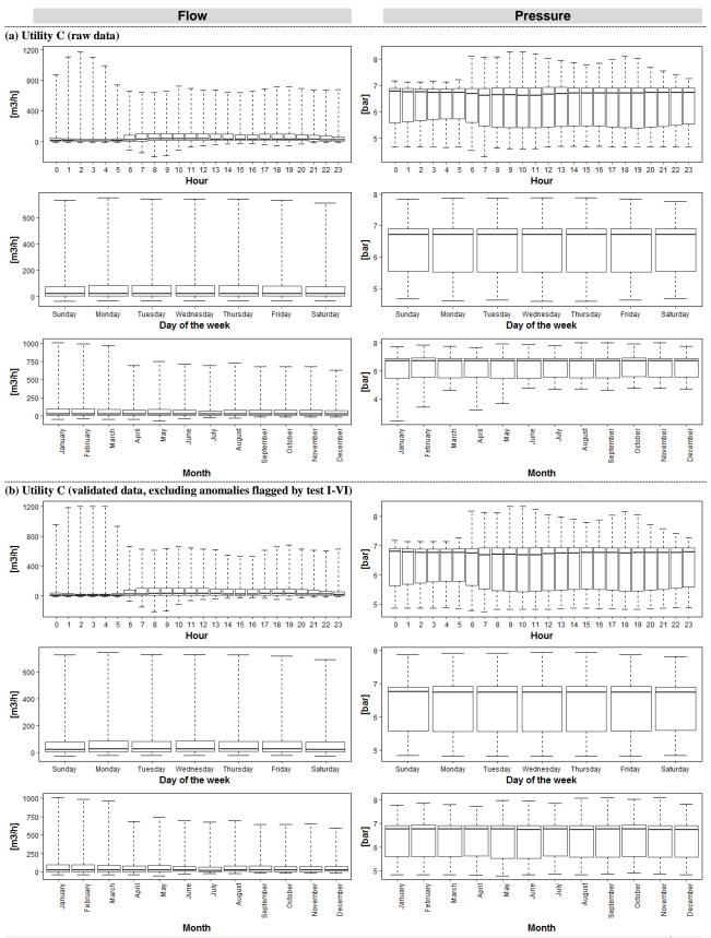
**Figure C-6.** Summary of raw (a) and validated (b) data sets in Utility C. Upper and lower hinge and whiskers represent the 25<sup>th</sup>, 75<sup>th</sup>, 2.5<sup>th</sup> and 97.5<sup>th</sup> percentiles. The line across the box displays the median. Except non-numeric values, no outliers have been removed from the raw data analysis. All values below the 2.5<sup>th</sup> and above the 97.5<sup>th</sup> percentiles are not displayed.
