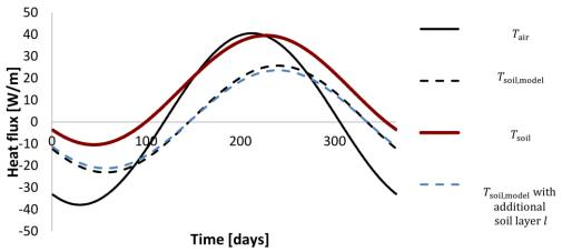
**Figure 16.** Heat flux per unit pipe length when the three temperature curves in Fig. 6 ( $T_{air}$ ,  $T_{soil}$  and  $T_{soil,model}$ ) are applied as input, and when (in a fourth case) an additional fictitious soil layer is added to the heat transfer model (blue, dotted). The inner pipe diameter is 0.2 m, and the pipe material is cast iron. The water temperature is 9 °C, and the water flow rate is 10 L/s.
