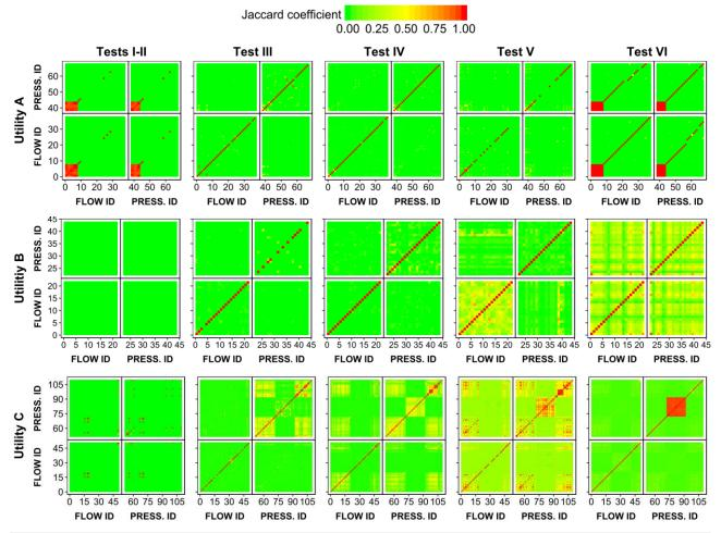
**Figure F-1.** The Jaccard coefficient computed for six different tests from the anomaly testing, based on the available flow and pressure meters. A Jaccard coefficient between zero and one describes no and very high similarity respectively for the occurrence of flags in the applied tests. Test types: I – duplicate timestamp, II – illegitimate timestamp, III – range, IV – rate of change, V – flatline and VI – timestamp inconsistency.
