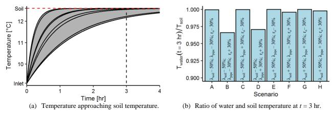
**Figure 4.** (a) Each line illustrates the change in water temperature of stagnant water in service lines over time based on the parameter scenarios listed in Table 3. Here, the initial water temperature was set to 9.1 °C and the soil temperature was set equal 12.6 °C. (b) Illustrates the water to soil temperature ratio after 3 hours. Remaining scenarios from Table 3 are listed in SI A.
