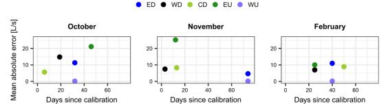
**Figure 7.** Days since last calibration of in-sewer sensors compared to the difference between observed flow  $(Q_{obs})$  and simulated flow  $(Q_{sim})$  calculated as the mean absolute error for the three time periods.
