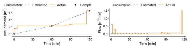
Figure 2. Linearly 'estimated' consumption over time based on two hourly measurements vs. actual consumption.
