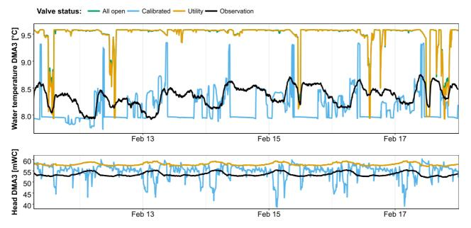
**Figure 9.** Temperature and head at DMA3 modeled for three valve scenarios. All valves open (green); a calibration with a weighting factor of 100% temperature measurements (blue); with the utilities knowledge of opened and closed valves (yellow); and the measured temperature at the location (black). Also, the measured and modelled head at the location are shown in the lower figure.
