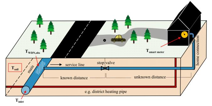
Unfortunately, smart meter temperatures ( $T_{smart meter}$ ) do not directly represent WDN temperatures, as the water temperature is influenced by various factors on its way to the consumer (Figure 1).
