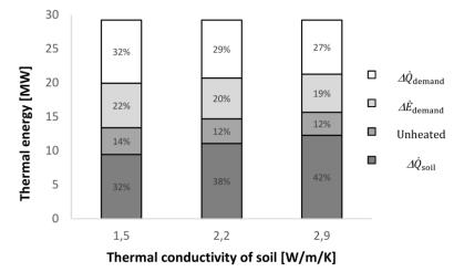
**Figure 15.** Heat utilization at different thermal conductivities of soil. The full height of each bar is  $\dot{Q}_e$ , the energy extracted from the water supply. The sum of the grey bar elements is  $\dot{Q}_{net}$ , the heat utilization from drinking water in the DH system; and their share of the full bar height is  $\eta_{util}$ . The percentage label on  $\Delta \dot{Q}_{soil}$  is  $\eta_{util,soil}$ .
