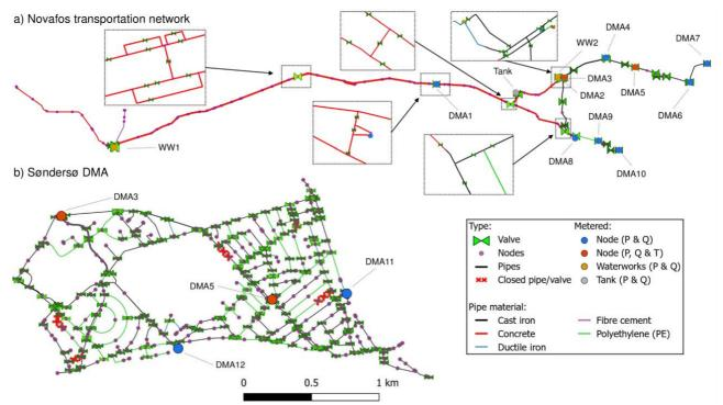
**Figure 4.** Novafos transportation water distribution network model. Lighter valve colours represent a higher number of overlapping valves. A close-up of the area around WW2 is illustrated in Figure 10b. WW = waterworks; P = pressure; Q = flow; T = temperature.
