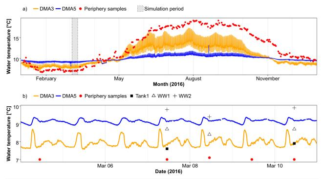
**Figure D-2.** Measured water temperatures at DMA3 and DMA5 including samples taken at WW1, WW2 and Tank and samples taken at the periphery of Copenhagen water distribution network assumed representative for the soil temperature.
