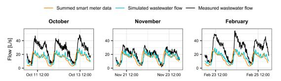
**Figure 8.** Observed sewage flow ( $Q_{obs}$ ) compared to simulated flow ( $Q_{sim}$ ) and summed smart meter data ( $Q_{SM}$ ) for three days in each of the three time periods for the 'CD' catchment.
