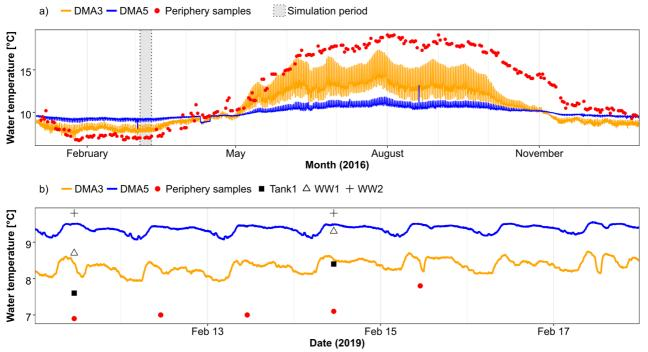
**Figure 5.** Measured water temperatures at DMA3 and DMA5 including samples taken at WW1, WW2 and Tank and samples taken at the periphery of Copenhagen water distribution network assumed representative for the soil temperature. The analysed period of March 2016 is illustrated in SI D.
