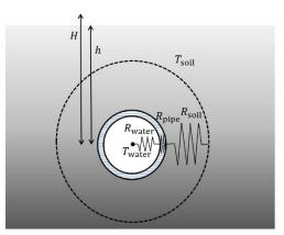
Figure 2. Thermal resistances, temperatures and correction terms included in the model [21, 22].
