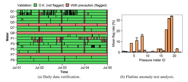
**Figure 6**. Example of anomaly visualisation for operational use. (a) Raw meter data validation from ten flow (Q) and ten pressure (P) meters in July 2015. (b) Mean flag rate based on all raw data points for the flatline test in pressure meters. Whiskers display the total flag rate based on all anomaly tests in the individual pressure meter, highlighting that flatline anomalies are the major anomaly source. From supporting information, Paper II.
