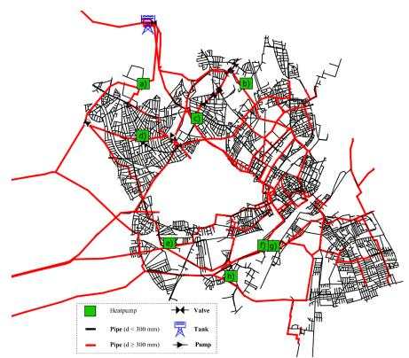
**Figure 4.** Locations of modelled heat pumps on the water distribution mains (red). Heat pumps f) and g) are located in low-temperature DH zone, while the other heat pumps are located in high-temperature DH zones.
