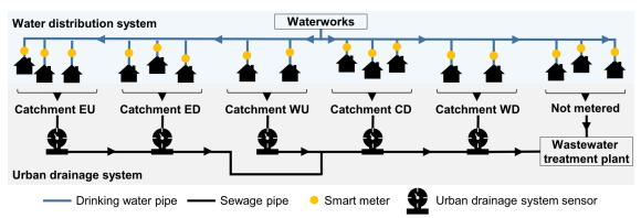
**Figure 12.** Linkage between a water distribution system with smart meters deployed and an urban drainage system consisting of five catchments. In-sewer sensors were installed downstream of these five catchments. Utility Elsinore, Denmark (Paper VI).
