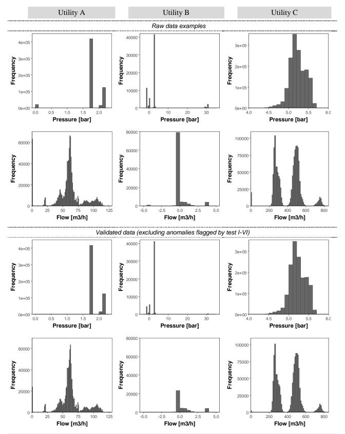
**Figure C-3.** Flow and pressure data histograms from six selected meters in utility A-C before and after data validation. Owing to the selected histogram bin size and margins, a minor share of data is not shown at maximum 0.06% (in this case raw pressure data in utility C).
