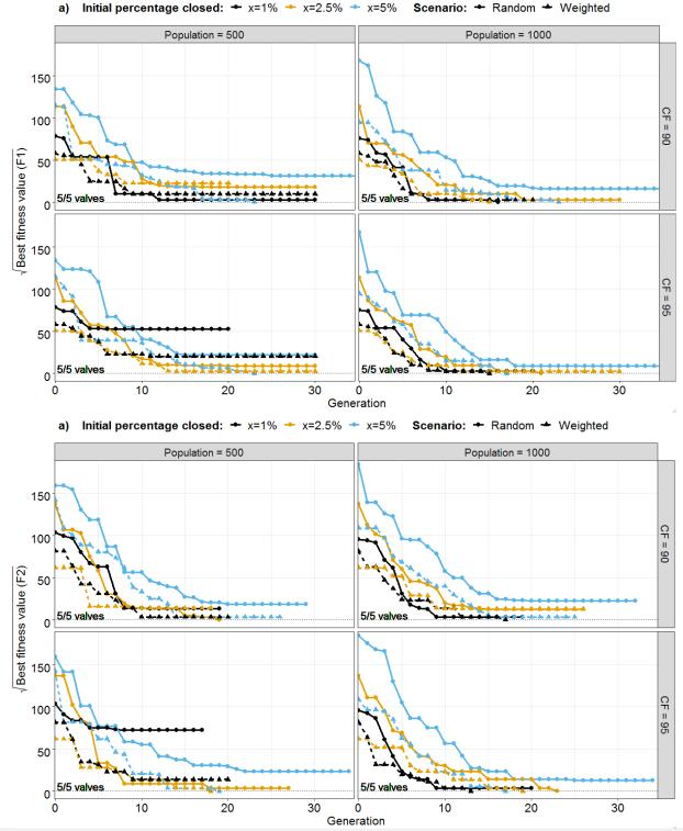
**Figure E-1.** Best fit of DMA model with various genetic algorithm (GA) set-ups; a) shows the GA runs with fitness function  $F_1$ ; and b) the GA runs with fitness function  $F_2$ . CF = Cross-over fraction. MR = mutation rate.
