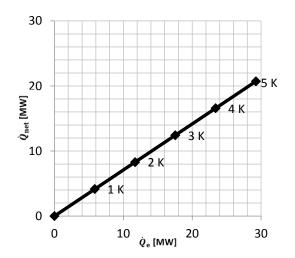
Figure 10. Potential for heat utilization  $(\dot{Q}_{net})$  vs. heat extraction  $(\dot{Q}_e)$ . The temperature reduction of the source is shown.
