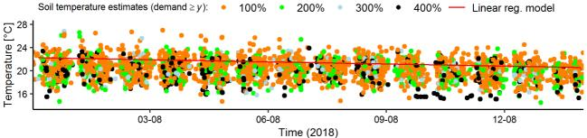
**Figure B-1**. Smart meter temperatures representing the water temperature in the water distribution network at different demand rates of *y* based on the filtering rules set in Table B-1.
