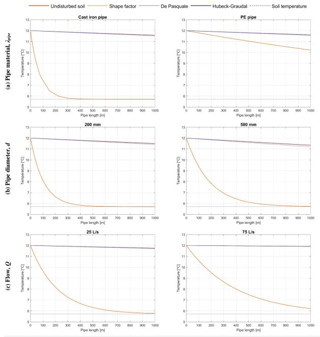
**Figure A-1**. Temperature profile of four different temperature models based on different set-ups, inspired by De Pasquale et al. (2017). For individual parameters of each set-up, see Table A-2.
