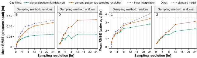
**Figure 6.** Mean root mean square error (RMSE) of pressure head (a–b) and water age (c–d) simulations with varying sampling methods and sampling resolutions based on all nodes with smart meters installed.
