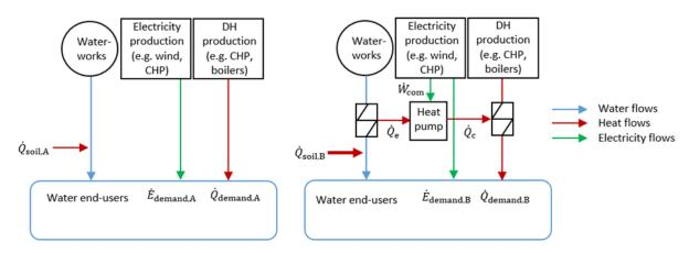
Figure 1. Energy system model without (A) and with (B) drinking water heat pumps (inspired by [11]).
