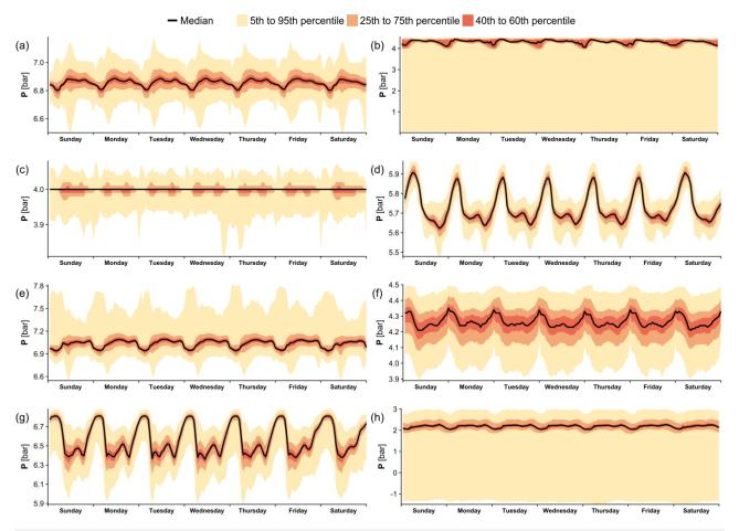
Figure C-2. Example of eight pressure time series applied in the case study. The percentile distribution is based on having grouped all measurements into a week's 168 hours.
