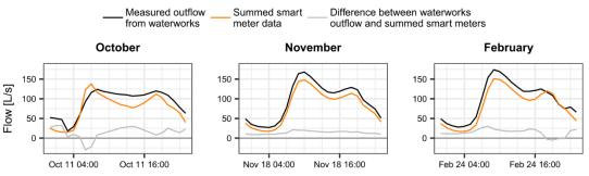
**Figure 2.** Hourly outflow data from the waterworks ( $Q_{WW,obs}$ ) compared to summed smart meter data ( $Q_{SM,Elsinore}$ ) for entire Elsinore (beyond what is shown in Figure 1) for single days in the three time periods.
