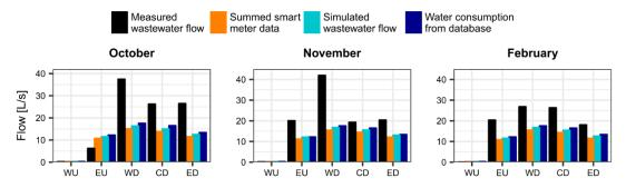
**Figure 4.** Average observed flow  $(\overline{Q}_{obs})$ , summed smart meter data  $(\overline{Q}_{SM})$  and simulated flow  $(\overline{Q}_{sim})$  (Eq. 2) in each of the three time periods compared to the average consumption from the water consumption database from 2012.
