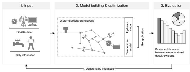
**Figure 1.** Overview of the four-step valve status identification process. GA = genetic algorithm; SCADA = Supervisory control and data acquisition.
