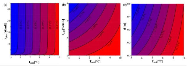
**Figure B-1.** Water temperature variation in the *Hubeck-Graudal model*, based on varying soil temperature and three parameters: soil conductivity ( $\lambda_{soil}$ ), pipe conductivity ( $\lambda_{pipe}$ ), and pipe diameter (*d*). Standard test set-up parameters are listed in Table A-1.
