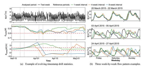
**Figure 4.** Example of a drifting flow meter in utility A. (a) The upper row displays the measured flow over time. The second and third row illustrate the computed correlation values  $[C_{weekly}(d)]$  and  $[P_{weekly}(d)]$  based on the applied test and three reference weeks needed in test VII. The drift is visible in (b) where the reference weeks are plotted against the test week at three selected periods.
