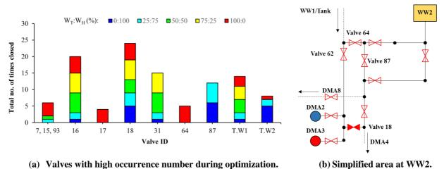
**Figure 10.** (a) The total occurrence of valves that have been closed at least once in more than 50% of the time of a given weighting scenario. (b) A simplified version of the network around valve 18, 64 and 87.
