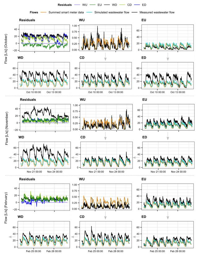
**Figure 6.** Summed smart meter data  $(Q_{SM})$  and simulated  $(Q_{sim})$  and observed  $(Q_{obs})$  sewage flows in October (top panel, Mon-Sat), November (middle panel, Mon-Sun) and February (lower panel, Sat-Fri) (Eq. 1). All data is in local time and  $Q_{sim}$  and  $Q_{obs}$  are displayed with a 30 minutes moving average filter to be able to distinguish graphs. Notice the different scales used for 'Residuals', 'WU' and the four remaining plots.
