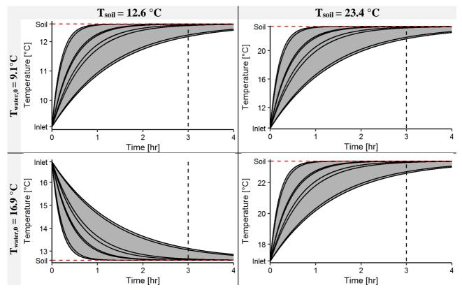
**Figure A-1.** Each line illustrates a parameter scenario (Table 3) leading to a change in water temperature of stagnant water in service lines over time.
