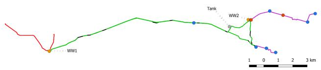
**Figure F-1.** Pipe segments not used for valve status identification, i.e. segments with no consumption and flow (dead ends), disconnecting consumers from a source and stretches clustered based on their proximity of 500m.
