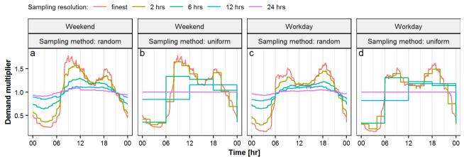
**Figure 3.** Generated DMA demand patterns, based on varying sampling methods and resolutions during  $01^{st}$  –  $15^{th}$  of August 2018.
