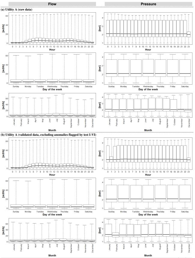
**Figure C-4**. Summary of raw (a) and validated (b) data sets in Utility A. Upper and lower hinge and whiskers represent 25<sup>th</sup>, 75<sup>th</sup>, 2.5<sup>th</sup> and 97.5<sup>th</sup> percentiles. The line across the box displays the median. Except non-numeric values, no outliers have been removed from the raw data analysis. Values below the 2.5<sup>th</sup> and above the 97.5<sup>th</sup> percentiles are not displayed.
