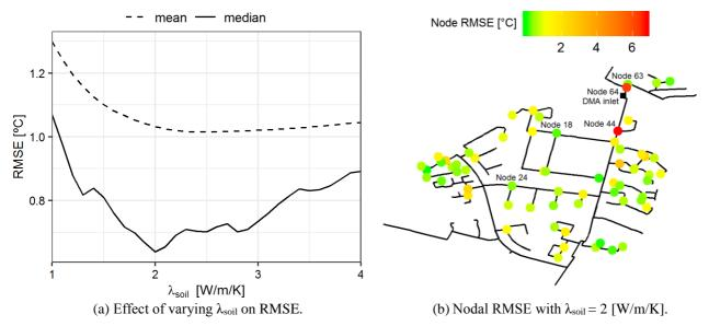
**Figure 7.** Varying the thermal conductivity of the soil ( $\lambda_{soil}$ ) affects the mean and median root mean squared error (RMSE) of all nodes in the analysed network (a). The nodal RMSE for  $\lambda_{soil} = 2$  [W/m/K] is illustrated in (b).
