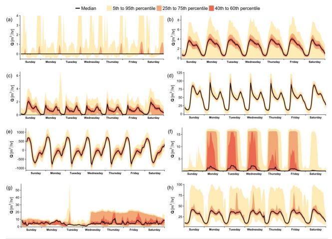
Figure C-1. Example of eight flow time series applied in the case study. The percentile distribution is based on having grouped all measurements into a week's 168 hours.
