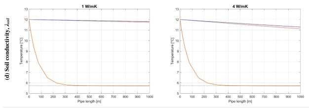
**Figure A-2**. Temperature profile of four different temperature models based on different set-ups, inspired by De Pasquale et al., (2017). For individual parameters of each set-up, see Table A-2. In (d), no  $\lambda_{soil}$  is included in the undisturbed soil model.
