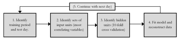
**Figure B-1**. Daily meter data reconstruction process based on artificial neural network models.
