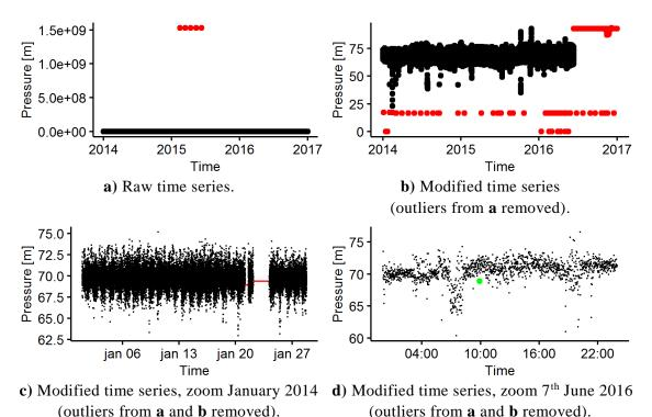
**Figure 4**. Example of pressure time series (• measurement • anomaly • control) collected at a district metered area outlet in Denmark.
