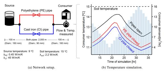
**Figure 8.** Modelled temperature variation when closing a polyethylene (PE) or unlined cast iron (CI) pipe, or having both pipes open. Based on the temperature model described in Paper IV.
