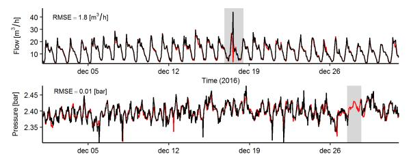
**Figure 7.** Measured (—) and reconstructed (—) pressure and flow time series from two Danish utilities. See Appendix B for more information. RMSE = root mean square error.
