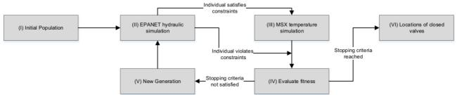
Figure 3. Concept for the genetic algorithm application to identify closed valves in a water distribution network model.
