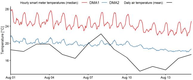
**Figure 3.** Temperature variation from 1,105 smart meters in two DMAs covering two weeks in 2018 and the daily mean air temperature from (DMI, 2019).
