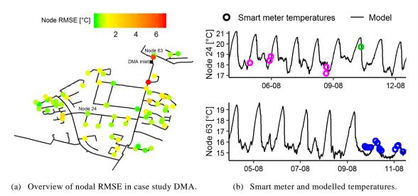
**Figure 10.** Examples of temperature variation throughout the case study water distribution network (Paper IV). (a) Nodal root mean square error variation (RMSE) based on temperature model and smart meter temperatures. (b) Example of two nodes with an RMSE of 0.36 °C (upper panel) and 0.32 °C (lower panel) where distinct colours represent individual homes' smart meters.
