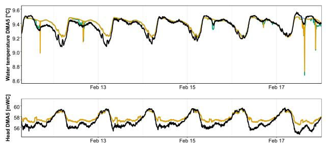
**Figure G-1.** Temperature and head at DMA5 based on various valve scenarios. All valves open (green); the model has only been calibrated with a weighting factor of 100% temperature measurements (blue); with the utilities knowledge of opened and closed valves (yellow); and the measured temperature at the location (black). Also, the measured and modelled head at the location are shown in the lower figure.
